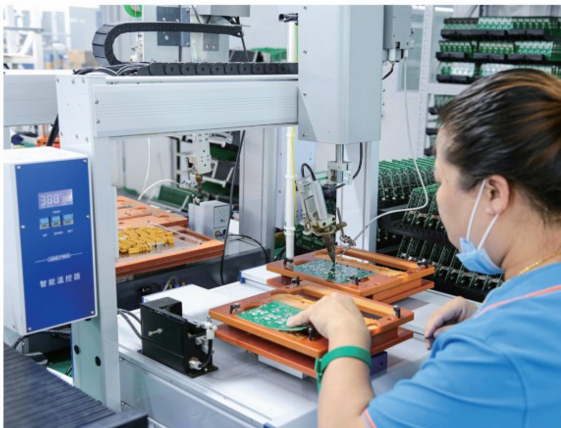
焊接机 Welding machine
